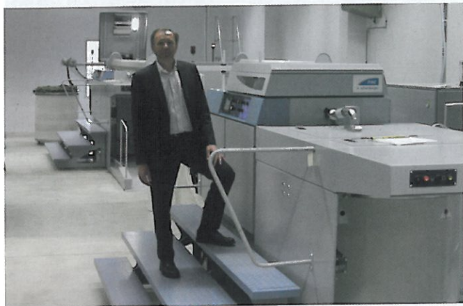
Patrick Strehle and a GC30 chain gill in the NSC fibre to yarn showroom specifically designed for customers to view completely assembled machines, see them running, and even enable them to test process their wool to see the end result and quality
