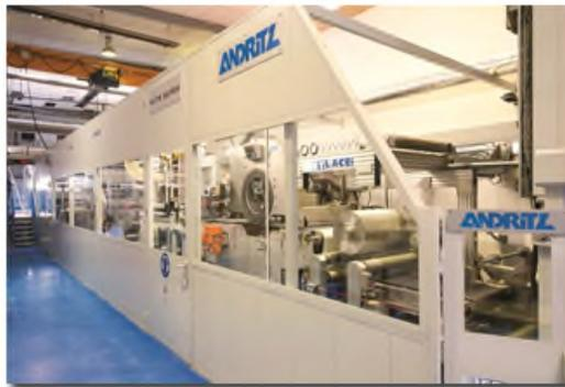
**Andritz Perfojet recently opened a laboratory facility equipped with a neXline spunlace pilot line for the production of hydroentangled nonwovens.**
