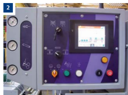
Man/machine dialogue at the control panel via a touch type screen terminal giving access to the functions of recording, speedometer, display, adjustment and help in diagnosis.
