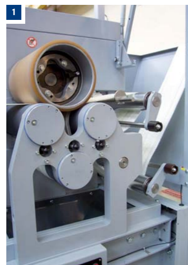
Feeding by up to 2 tows with safety in case of overloading and overtension.
